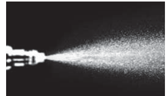
Injector spray pattern after P.i. treatment.
