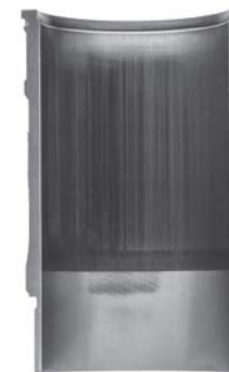
Severely Scuffed Liner
